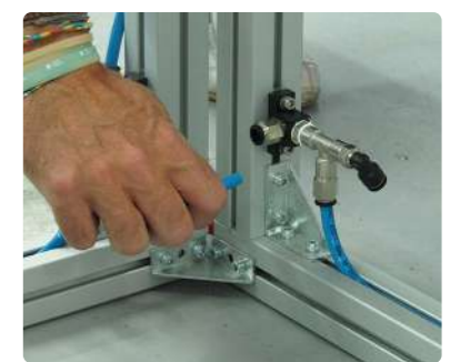
Connect Air connection pipes
