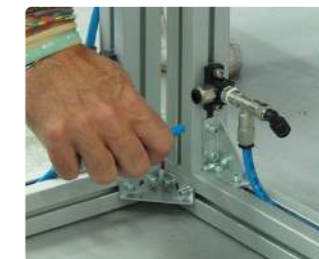
Connect Air connection pipes
