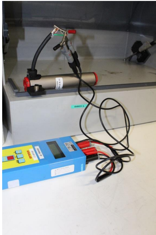
Fig. 11. - Photograph set-up for Insulation resistance test
