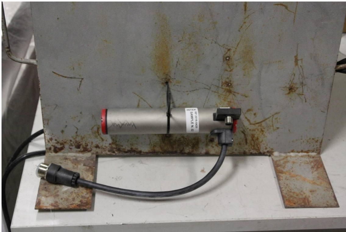
Fig. 7. - Photograph set-up for IPX7 test
