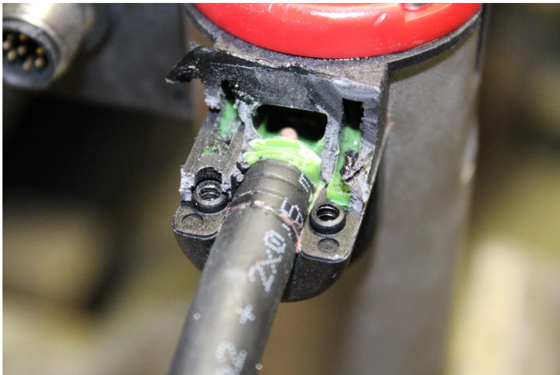
Fig. 8. - Photograph result after IP67 Test
