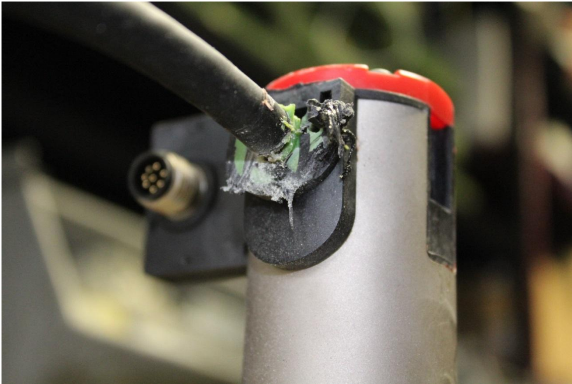
Fig. 9. - Photograph result after IP67 Test
