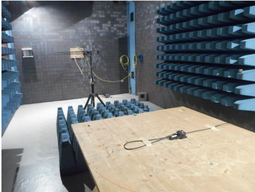
Photo of the test set-up for frequency up to 1 GHz
