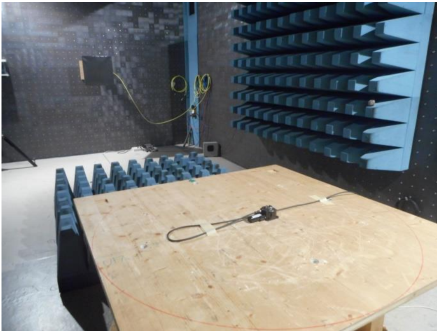
Photo of the test set-up for frequency above 1 GHz
